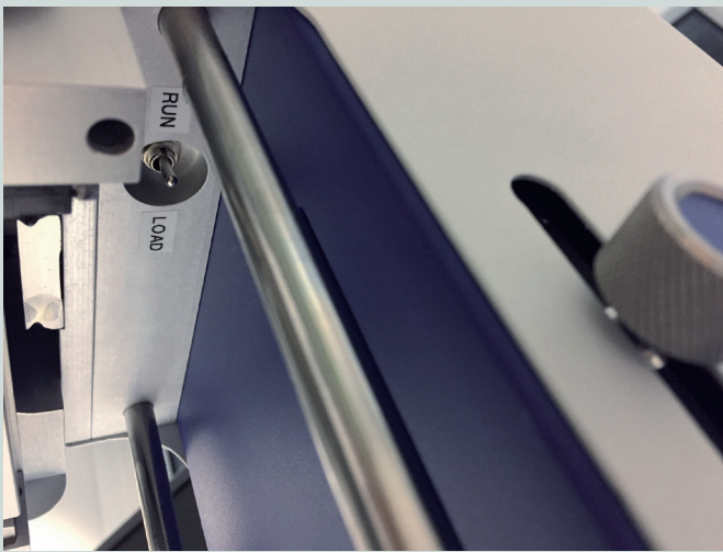
Figure 2: Switch for firmware updates can be found behind the tip loading frame below the pipetting head.
