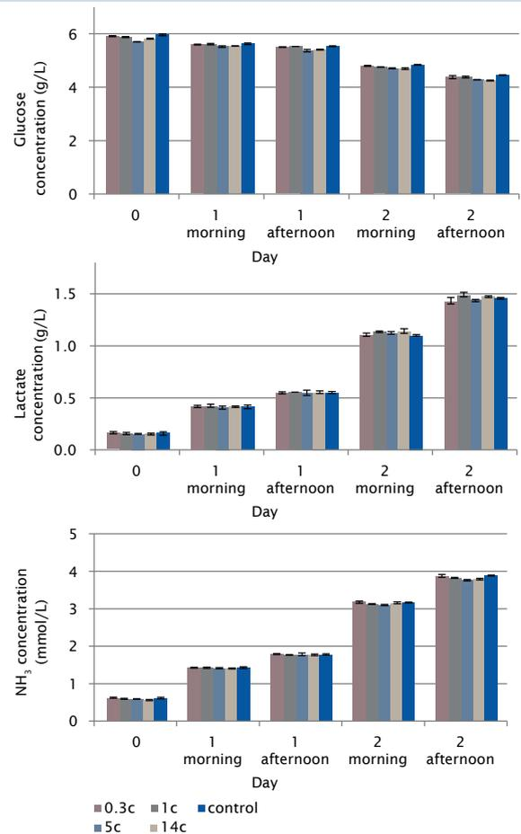
**Fig. 5:** Cell metabolism. CHO cells were cultivated in extraction media from BioBLU Single-Use Vessels or a shake flask (control) and substrate (glucose) and metabolite (lactate, NH<sub>3</sub>) concentrations were measured twice daily.
