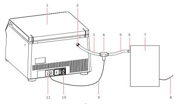
Figure 4: Connecting a vacuum pump<sup>1</sup> with > 400 W power consumption to the Concentrator plus basic device.
