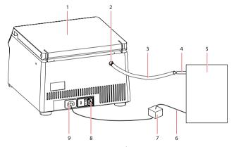
Figure 2: Connecting a vacuum pump¹ with < 400 W power consumption to the Concentrator plus basic device
