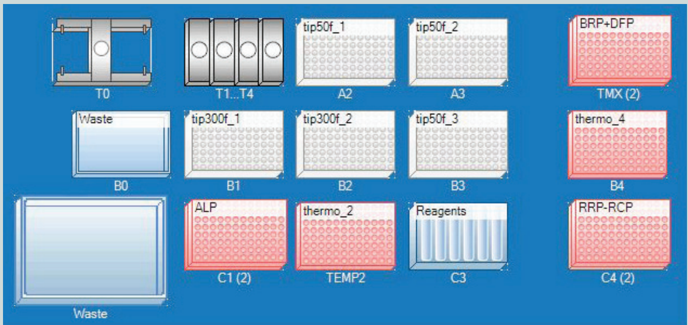
Figure 2: epMotion worktable layout for method 1
