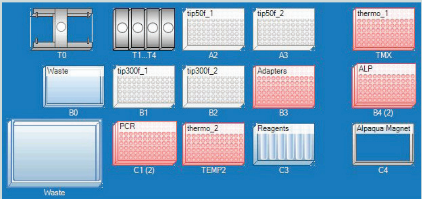
Figure 4: epMotion worktable layout for method 2
