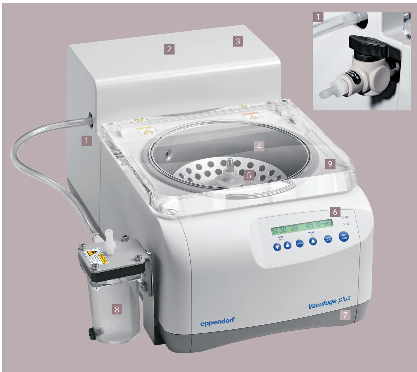
**1** Optional vacuum port adds extra flexibility. Allows for connecting external devices to the vacuum pump.
