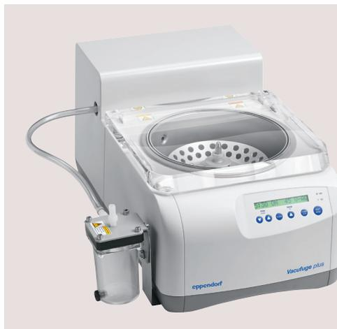
Complete System with an integrated solvent-resistant, maintenance and oil free PTFE pump, and condensation trap. Condensation trap purifies exhaust air by up to 85 %, protecting against unpleasant vapors. At the same time, it extends the service life of all components that come into contact with the vapors.
